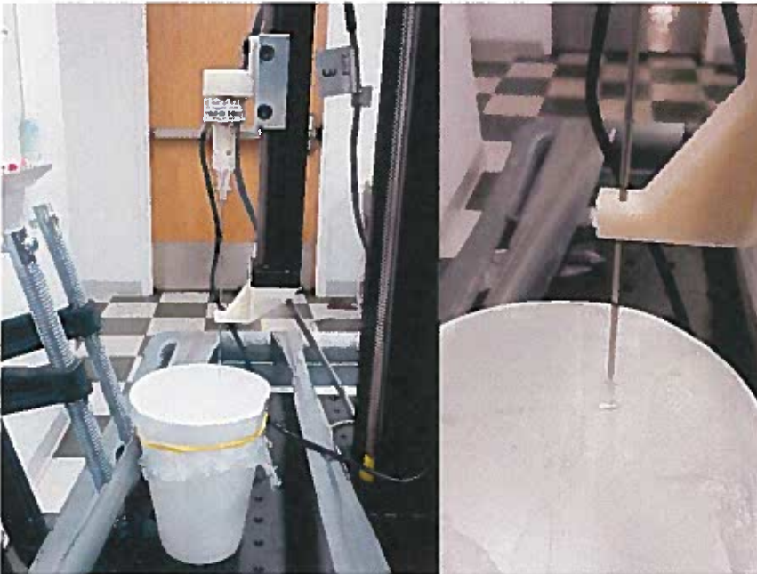
Figure 8. Needle insertion test set up for polyacrylamide cubes.
