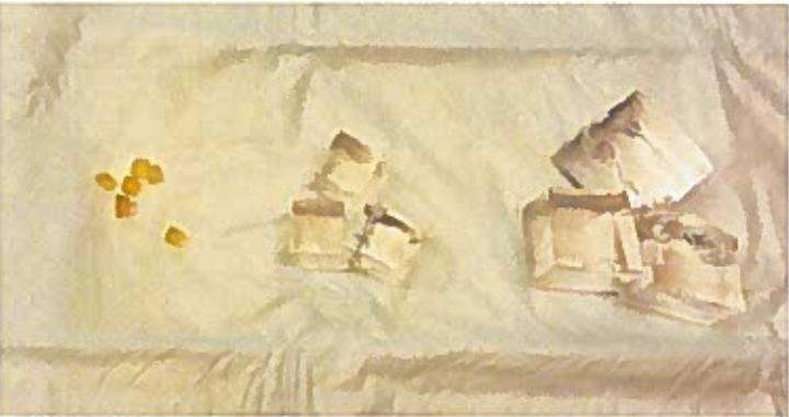
Figure 6. Initial, intermediate and final sizes of polyacrylamide cubes after being placed in distilled water.
